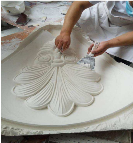
Figure 4. Modification of GRG's unique module.
