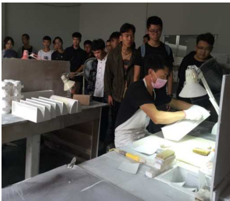
Figure 5. Modification and quality inspection GRG module.
