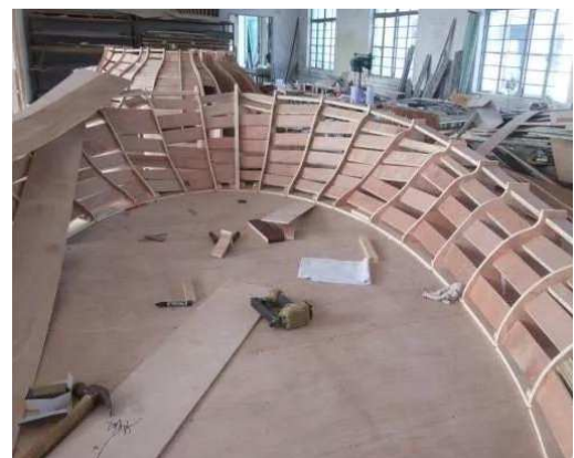
Figure 3. Wooden mold of prefabricated GRG module.
